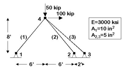
The example demonstrates a typical finite element exercise by representing a truss configuration using nodes, elements, materials, loads and constraints. Model:
