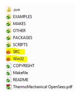
The two main folders of interest for OpenSees development are **SRC** and **Win32**. The SRC folder contains the source scripts and the files in win32 control the source codes in SRC. The source files (\*.cpp) and the header files (\*.h) for individual projects can be found in the sub folders of SRC.
