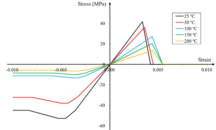
Material degradation of timber fibers
