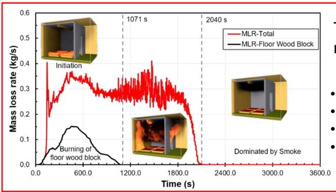
The fire development is simulated using a model in Fire Dynamics Simulator (FDS).
