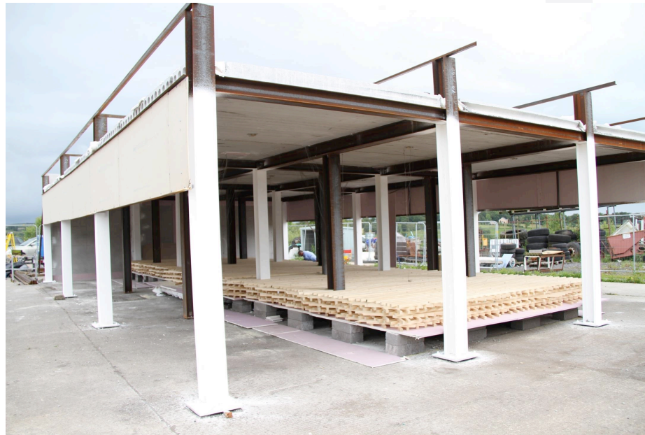
Experimental building and fuel bed layout of the TRAFIR-Ulster Travelling Fire Test 1
